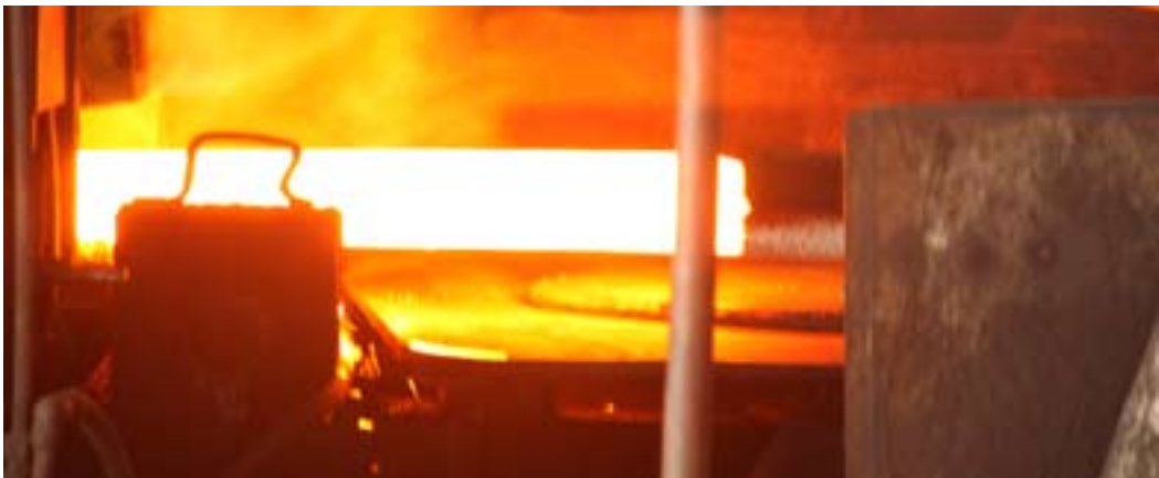
Hot billet after being ejected from the energy-efficient re-heating furnace
